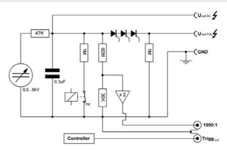
Schematic Diagram of the Probe Calibration Generator KHT 6000 C
